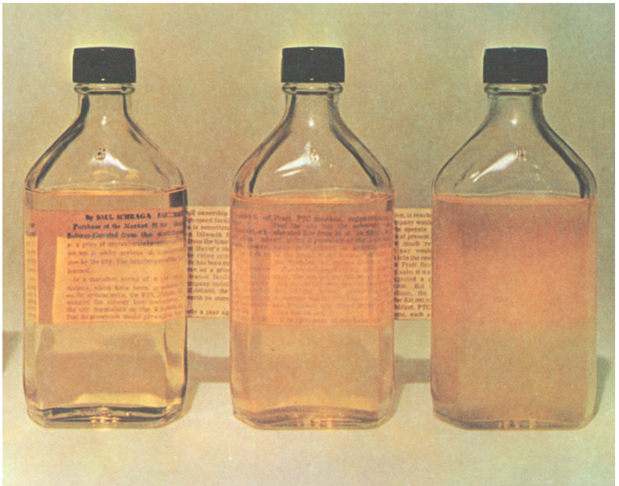
Figure 3-3.—Degrees of cloudiness in JP-5. The left sample is clean and bright and is the only acceptable fuel for aircraft.
